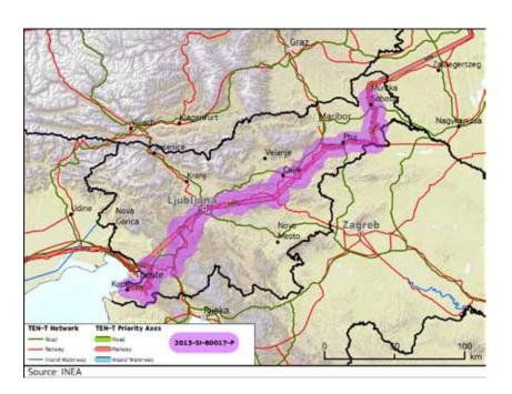
The proposed Action covers the deployment of ETCS level 1 version 2.3.0d with infill functionality on the entire Slovenian part of Corridor D. According to the proposal, the ETCS will be deployed on 292.95 km of rail and cover the entire line from the border to border (Hungary to Italy) with a connection to the Port of Koper. It follows a pilot project from 2013 and is in line with the country's national programme for railway infrastructure development.
