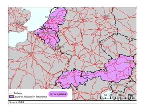
The proposed Action features the upgrade and retrofitment of ETCS 2.3.0d on-board units on 60 TRAXX locomotives and upgrade and retrofitment of 22 Vossloh G2000 locomotives with ETCS Baseline 3. The locomotives are currently used on parts of different rail freight corridors (1, 3 and 8) as well as Priority Project 17 (Railway axis Paris-Strasbourg-Stuttgart-Wien-Bratislava).
